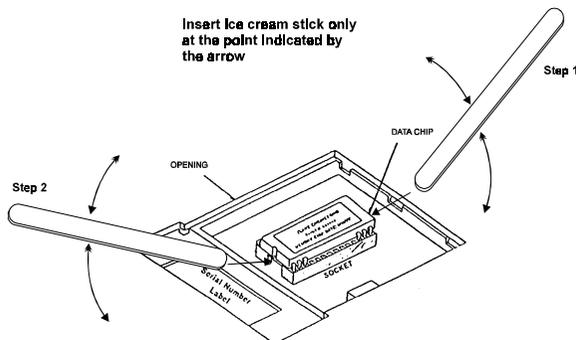
3. Align the NEW DATA CHIP on top of the chip carrier, so that the chip pins coincide with the corresponding holes in the DATA CHIP Socket. **Take care of the orientation of the Data chip and the Socket, the marked end of the Data chip should be towards the marked end of the Socket.**
