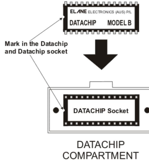
4. When the CHIP is sitting smoothly on top of the socket with each pin inside the corresponding hole, press NEW DATA CHIP with your two thumbs until it fits snugly into the Socket and replace the DATA CHIP COVER.
